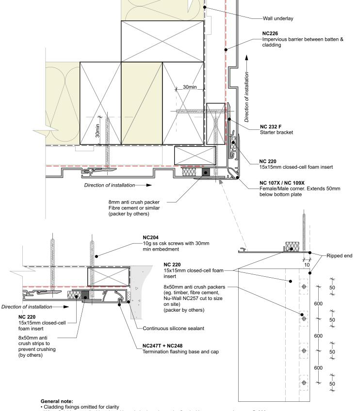
• When finishing a wall with a ripped board, the board must be fixed with a counter sunk screw @ 600mm centres
