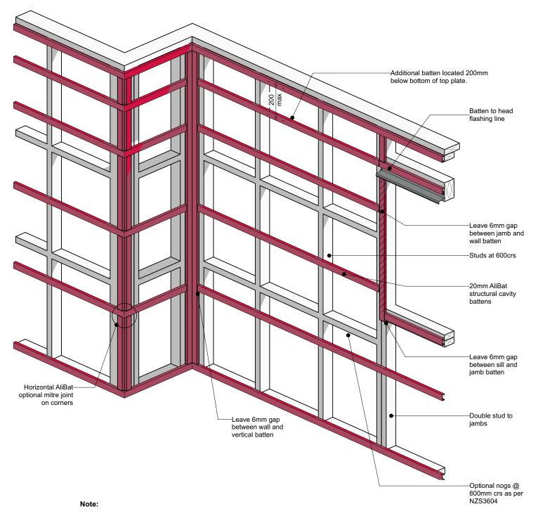
• Nogs are not required for Nu-Wall horizontal board installations when using AliBat
